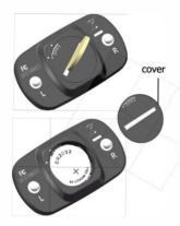
Remove the old battery and Insert the new battery into the cover, with the + (plus) side facing to the cover.
